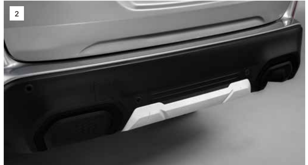
2 Rear Resin Under Guard E551ESL500
